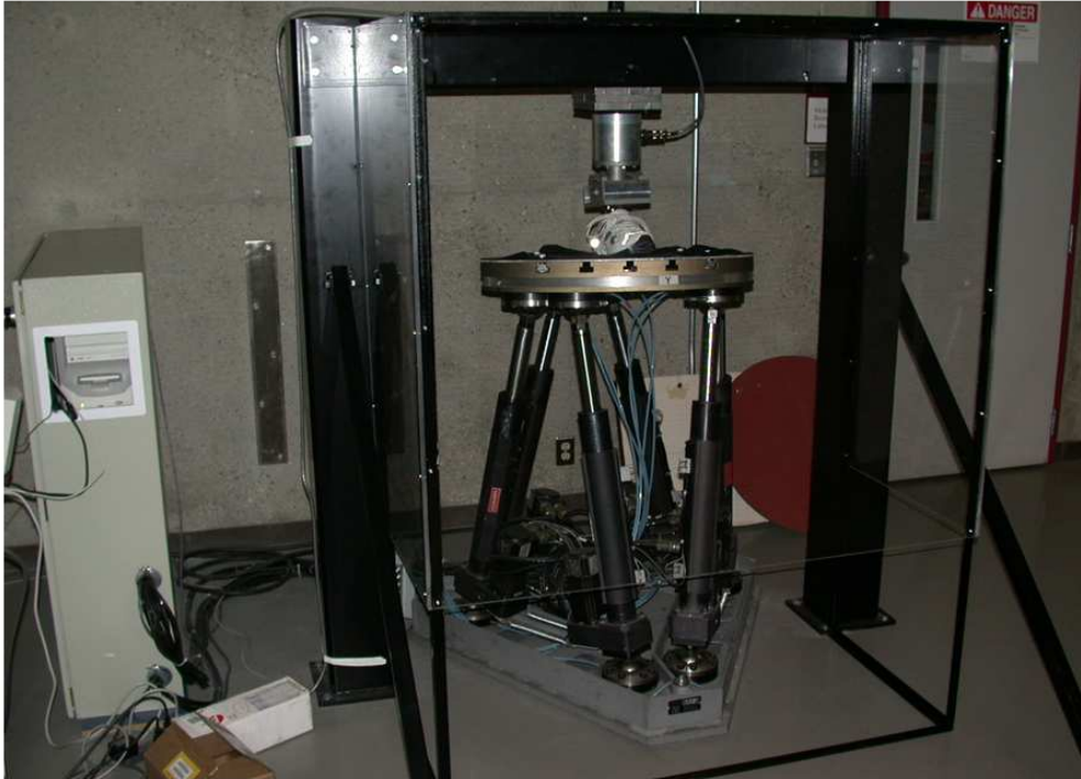
Figure 2.1: The Automated Foot Testing System consisting of the robotic Stewart platform, the prosthetic foot (shown here with shoe attached), the rigid frame, and the load cell (the cylinder just above the shoe).
